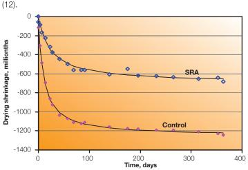
FIGURE 4. Drying Shrinkage of Concrete with and without MasterLife SRA 20.
