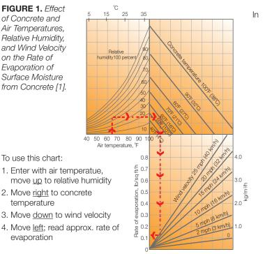
ACI 305R [2], it is recommended that precautions against plastic shrinkage cracking should be taken if the evaporation rate from the exposed concrete surface is expected to approach 0.2 lb/ft<sup>2</sup>/h (1.0 kg/ m<sup>2</sup>/h). The evaporation rate for a prevailing ambient condition can be estimated by using the nomograph shown in Fig. 1.
