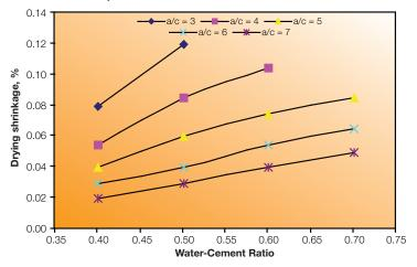
**FIGURE 3.** Effect of Aggregate-Cement Ratio (a/c) and Water-Cement Ratio on Drying Shrinkage [8]. (Data from 5 in. (125 mm) square mortar and concrete specimens exposed to a 70 °F (21 °C), 50 percent relative humidity environment for six months.)
